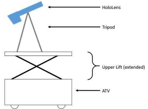
Fig. 2. ATV with extended LHD and tripod with mounted HoloLens.
