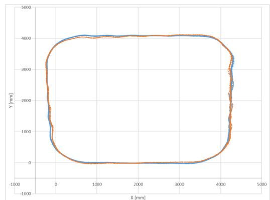
Fig. 4. Reference marker only at start (OptiTrack blue; HoloLens red).
