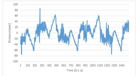
Fig. 12. Distance between OptiTrack and HoloLens after transformation - X-direction..
