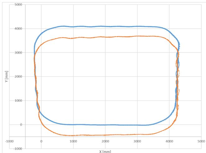
Fig. 11. Recorded data of Optitrack (blue) and non transformed data of HoloLens (red).
