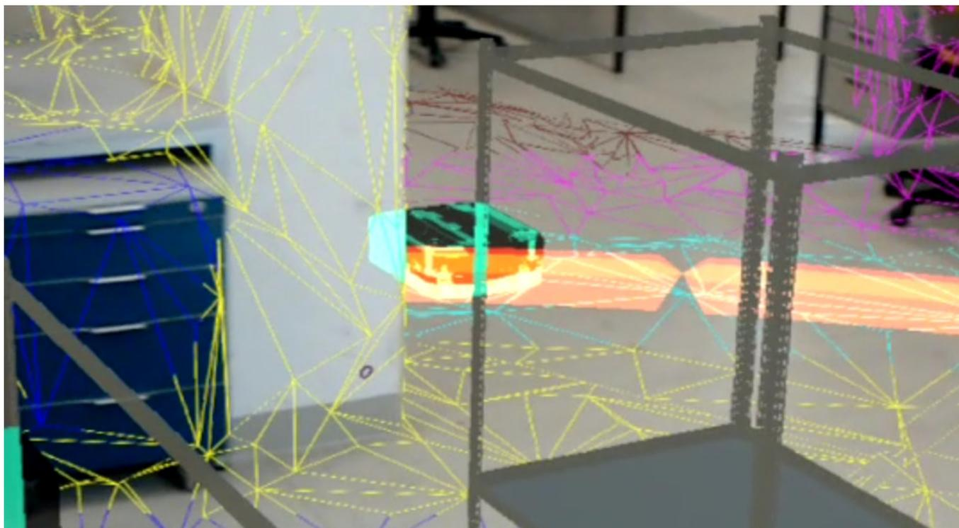
Figure 4: Occlusion of the robot both behind real obstacles and holograms.
