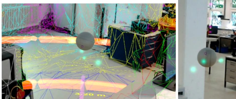
Figure 1: The line following on the left with incorporated distance to goal and the particle stream on the right (the pink particles above the spherical goal). The green particles were experimented as an additional way to make the goal more visible
