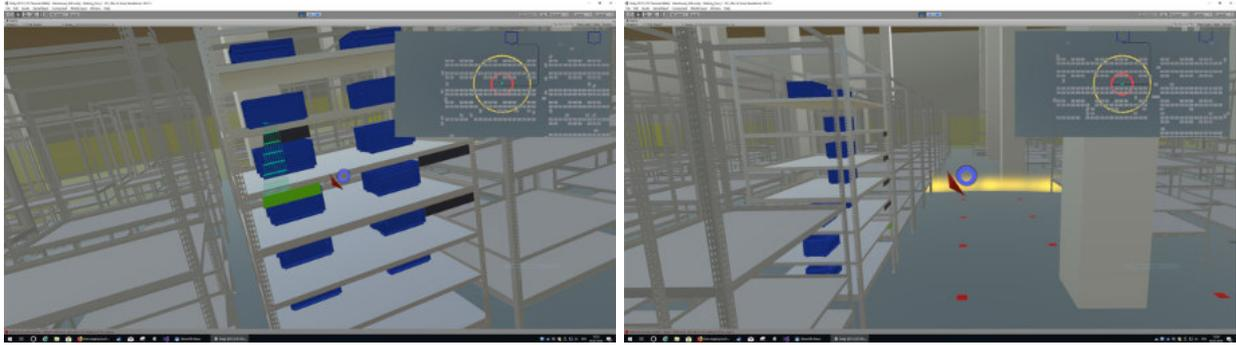
Figure 10: The picking assistance implemented in VR. Note that the FoV restriction for the Holograms still apply as on the Hololens. Also to note is the cut x-ray image of the robot on the left image. This is due to the robot just entering the visualisation zone.
