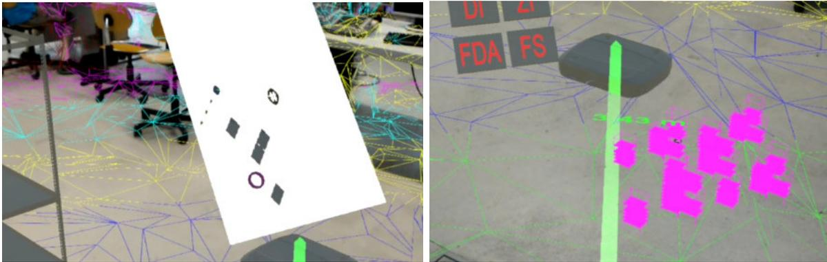
Figure 2: The 2D minimap on the left called from the menu. On the right the 3D minimap that automatically places itself on the floor in front of the user. Both minimaps can visualize robots, paths and allow a zoom in and out function
