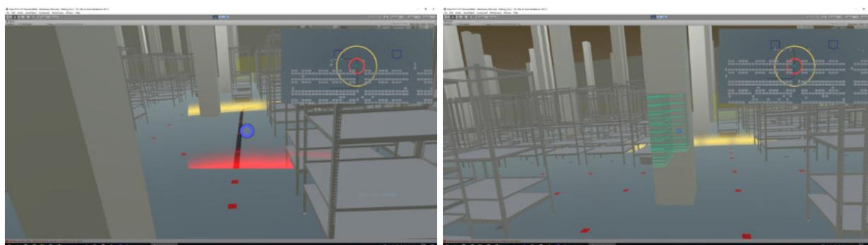
Figure 9: The two safety levels visualised and the line navigation on the ground on the left image. The x-ray vision of the robots on the right one. Note that the map in the upper right corner is not visible to the users although they can enter a top-down view - the same as on the hololens.
